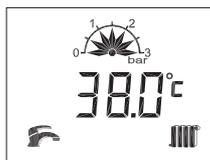
Heating and DHW heating enabled
