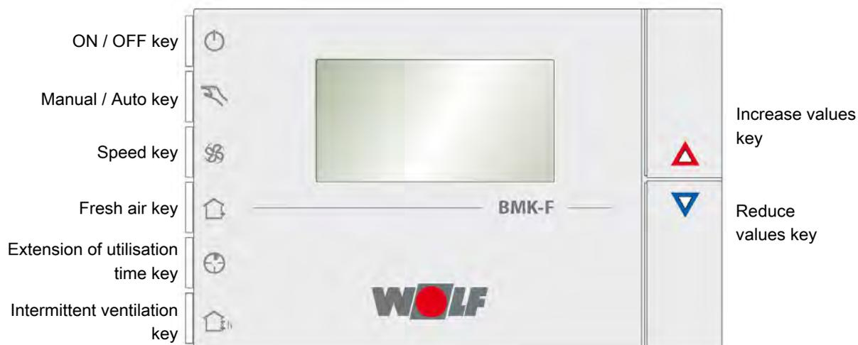
**ON/OFF key** The system can be switched on and off with the ON / OFF key. When the system is shut down, the indication “OFF” will be shown on the display instead of the set temperature. Special operating modes (back-up mode etc.) remain active.
